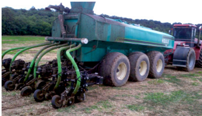
Figure 2. The 6,300 gallon tanker fitted with Dawn® injectors that was used in the economic assessment in the Shenandoah Valley.
