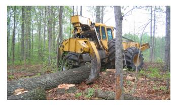
After trees are either felled with a piece of machinery or by hand with a chainsaw, they are typically moved to the log deck with a skidder, such as this "grapple"-style skidder that lifts one end of the log and drags the other.
